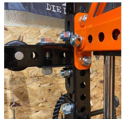
Connect different Brand 3x3 Uprights with a Bolt & Bracket Connected to Rouge Monster Upright & Bracket Connected to Stray Dog Upright
