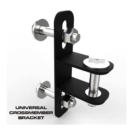
The Custom Crossmember Brackets are sold only in Pairs and were designed to allow customers to make a Crossmember at a custom length by pairing a 3×3 tube with and custom crossmember bracket. The slotted bracket allows customers to create a custom length crossmember to connect different brand 1" hole 3×3" racks or our ATR units to other brand racks. Each Bracket comes with the Hardware shown in the rendering. The price shown is for 2 brackets and bolt assemblies.
